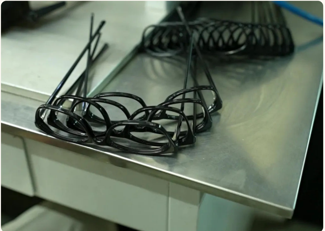
Core wire, before it is set into the temple — the part nobody photographs.
